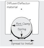
clamp should be pushed back against the front of the housing.
